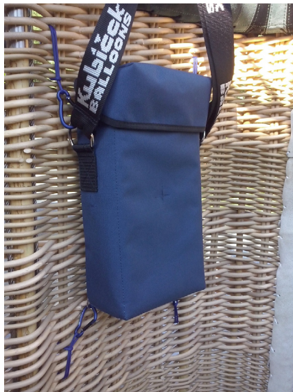
Installation of Storage Bag to Basket Wall
